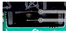
Install Battery Between These Two Points
